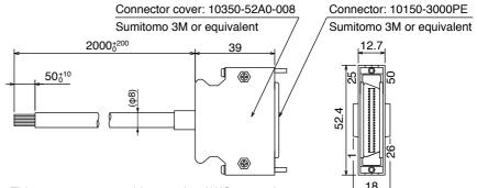
This 2 m connector cable contains AWG28 conductors.
