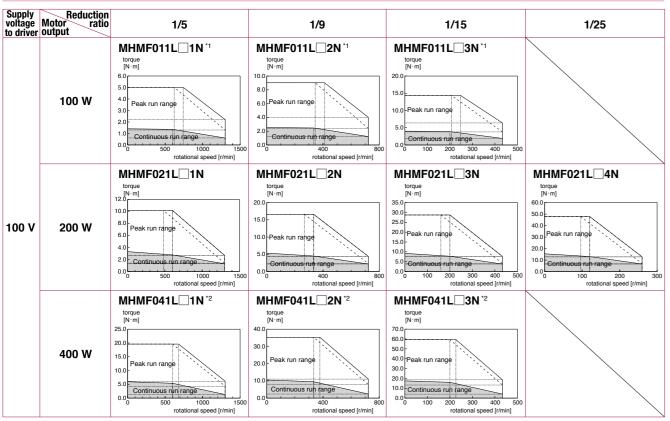
Dotted line represents the torque at 10 % less supply voltage to driver.
