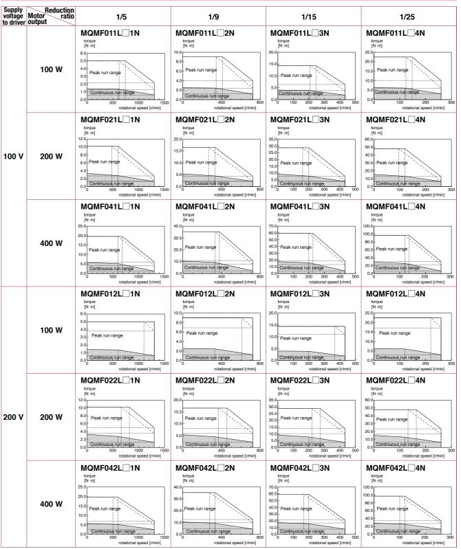
Dotted line represents the torque at 10 % less supply voltage to driver.
