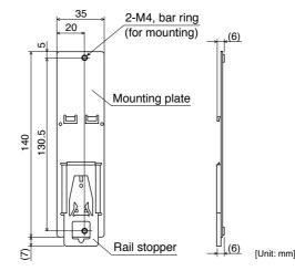
**DIN Rail Mounting Unit/ External Regenerative Resistor**
