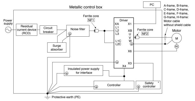
For NF1 to NF2, refer to the Table "Ferrite core" (P.414).
