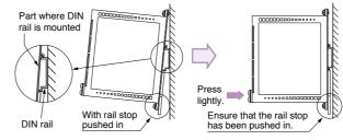
Hook the upper side of DIN rail Press lightly the lower part mounting part on the DIN rail. of the main body of driver.
