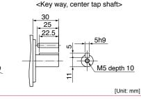
Mass: 1.6 kg Motor model Motor model No. Power supply Shaft Round MHMF041L1D4 100 V MHMF041L1V4 Key-way, center tap MHMF042L1D4 Round 200 V MHMF042L1V4 Key-way, center tap Dimensions are subject to change without notice. Contact us or a dealer for the latest information
