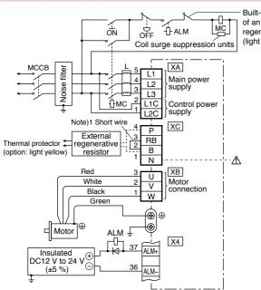
Built-in thermal protector of an external regenerative resistor
