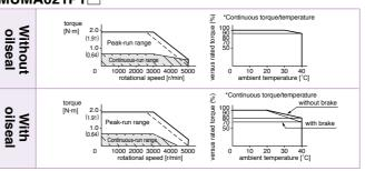
Running range (Torque limit setup: 100 %)
